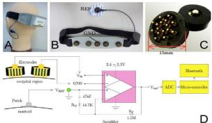
**Fig: 1.** Wireless and wearable EEG devices. (a) Wireless and wearable EEG headsets. (b) Five dry EEG electrodes and one patch sensor. (c) Spring-loaded probes. (d) Block diagram of the circuit
